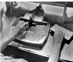
Pantograph for creating punched cards for the Tabulating Machine http://www.census.gov/history/img/pantograph.jpg
