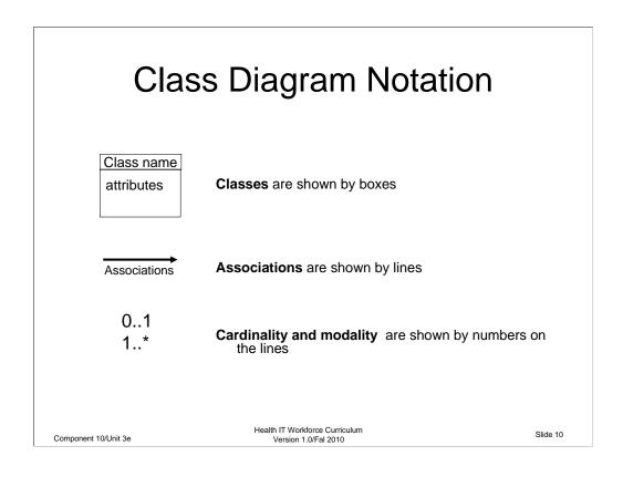
A class, shown by a box, represents the information collected, generated by or used in a process.
