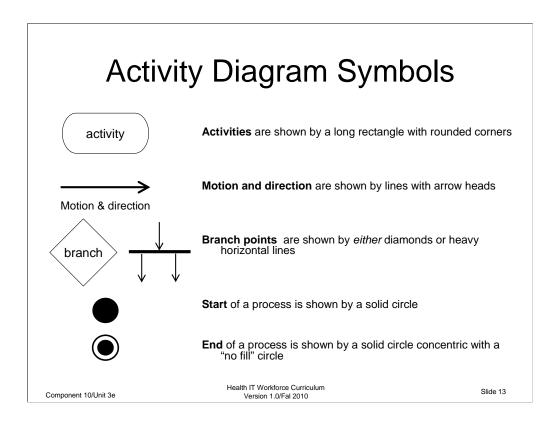
An **activity**, shown by a long rectangle with rounded corners, is a task that is performed either by a person or a computer system.
