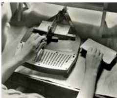
Pantograph for creating punched cards for the Tabulating Machine http://www.census.gov/history/img/pantograph.jpg
